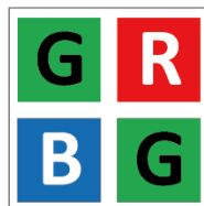
Figure 11-7 Bayer GR Pixel Pattern
