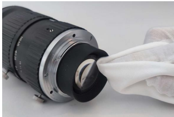
Figure 2-3 Cleaning by Lens Cleaning Paper
