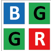
Figure 11-9 Bayer BG Pixel Pattern
