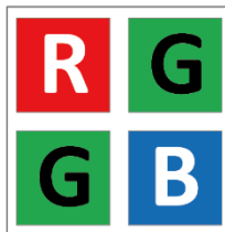
Figure 11-10 Bayer RG Pixel Pattern
